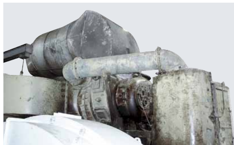
Engine 18V40/54 | 2 x VTR 401 replaced by 2 x NA34/S
