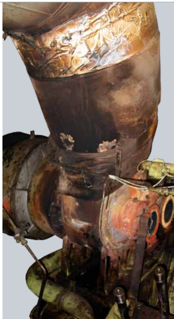
Engine 12V40/54 A | 2 x NA34/K replaced by 2 x NR26/R
