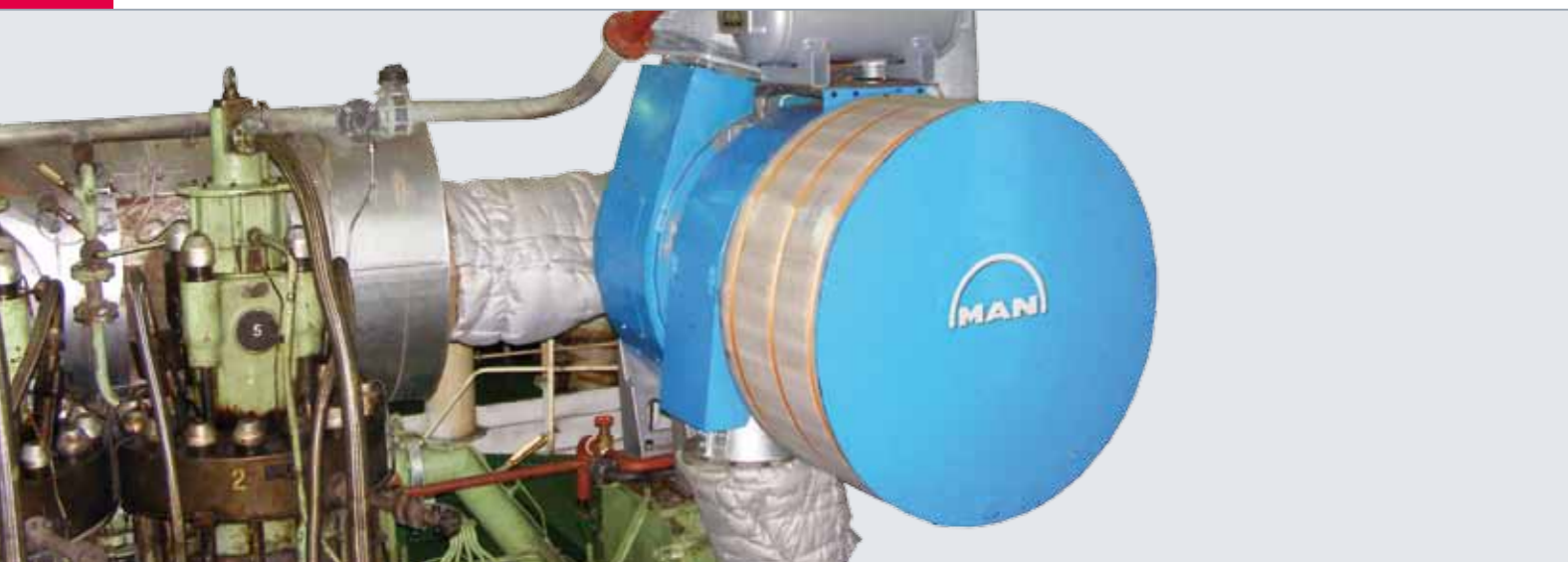
Engine 6S50MC | 1 x NA48/T replaced by 1 x TCA55
