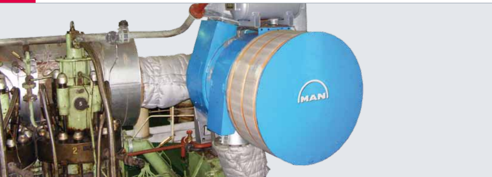
Engine 6S50MC | 1 x NA48/T replaced by 1 x TCA55
